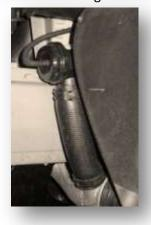
4. The original dumpvalve can now be removed. You can do this using pliers or using a special hose clamp pliers as shown in the picture below (on left). We found it easier to remove the vacuum hose first and then the one on the bottom port next (the one tucked away). Finally remove the hose on the side port.
