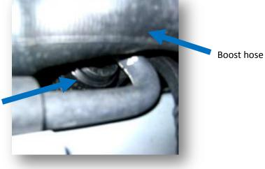
13. You will need to remove this hose so that you can gain access to the recirculation valve to change it. To do this pull the 'U' shaped circlip off. This can be done by prising it off with a flat blade screw driver. Slacken the hose clamp on the other side and pull the hose off using a flat head screw driver, hose clamp driver or 7mm socket. This will give you a better view of the valve.
