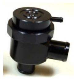
All products made by Forge Motorsport are quality controlled before being sent out, but we recommend that you carry out a check of the dump valve before fitment. This can be done by pushing in the piston at the bottom port of the valve and covering over the vacuum nozzle with your finger. Release your finger off the vacuum nozzle and the piston should drop back down and make a 'popping' noise. This proves that your valve is in working condition.
